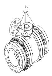
Wrong methods for Hoisting Ball Valve
