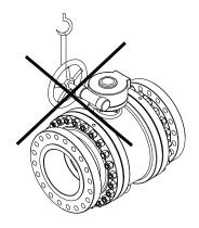
valve. Failure to do so may result in damage to the soft seats.
